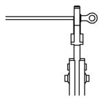
Use the crimping pliers to press the ground cable into the ground terminal, screw the ground screw with screwdriver as shown below:
