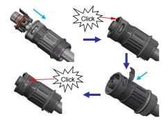
• Insert Seal and Clamp Finger into socket ,then tighten the nut , torque 8+/-2N·m.
