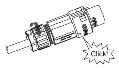
• Push the threaded sleeve to connection terminal until both are locked tightly on the energy station.
