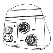
• Remove the ON-GRID connector: Press the bayonet out of the slot with a small screwdriver or the unlock tool and pull it out, or unscrew the threaded sleeve, then pull it out.
