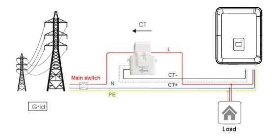
If there is another generator in the home, CT2 can be used to record the power generated by the generator and transmit the data to the website for monitoring.
