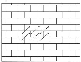
Insert the expansion tubes into the holes and tighten them. Install the bracket with the expansion screws.
