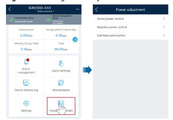
Figure C-1 Setting Power Adjustment Parameters
