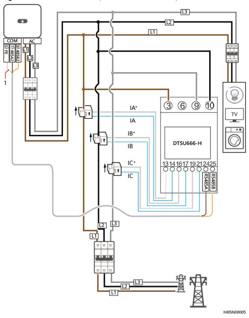
Figure 5-22 Cable connection (Three Phase Three Wire)
