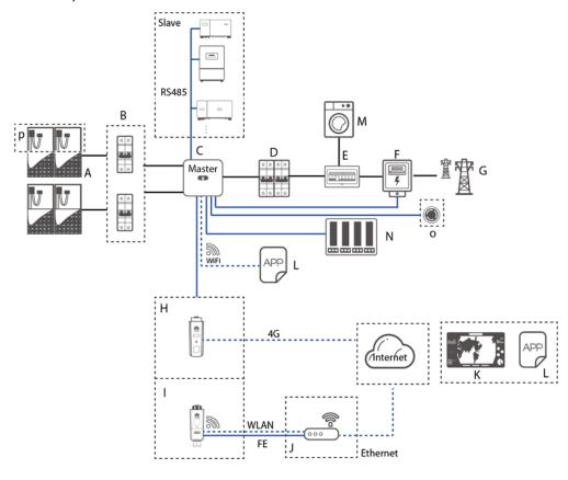
**Figure 2-3** Networking application - Inverter cascading scenario (optional in dashed boxes)
