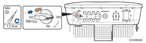
**Step 5** Turn off the DC switch between the SUN2000 and PV strings.
