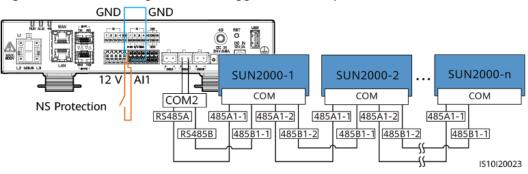
Figure 5-34 Connecting the SmartLogger to the NS protection switch
