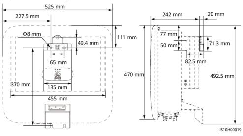
Figure 4-7 Mounting bracket dimensions
