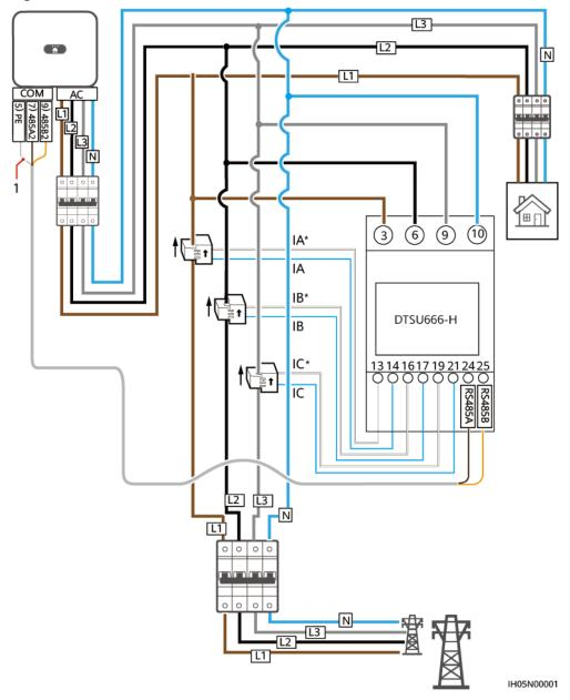
Figure 5-23 Cable connection (Three Phase Four Wire)
