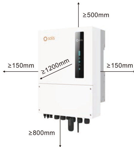
Figure 3.5 Inverter Mounting Clearances
