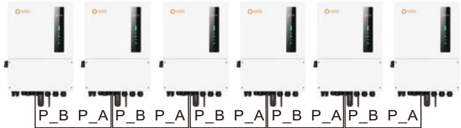
Figure 3.24 Parallel Terminal Connection
