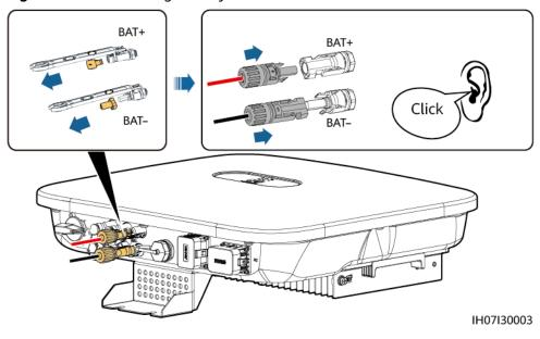
Figure 5-15 Connecting battery cables
