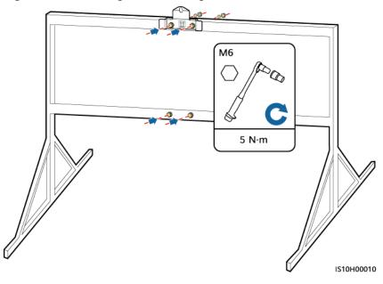
Figure 4-15 Securing the mounting bracket
