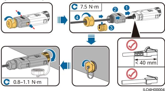
Figure 5-16 Installing a WLAN-FE Smart Dongle (FE communication)
