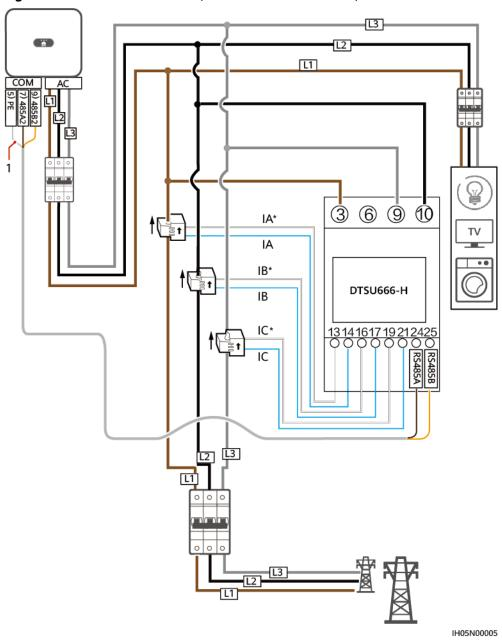
Figure 5-23 Cable connection (Three Phase Three Wire)
