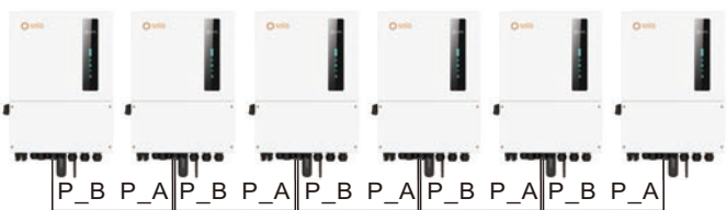
Figure 3.24 Parallel Terminal Connection
