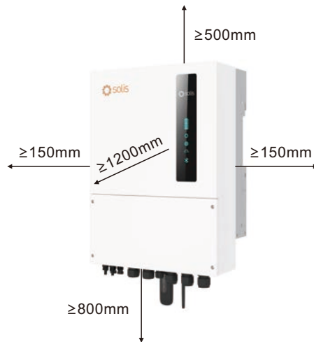
Figure 3.5 Inverter Mounting Clearances
